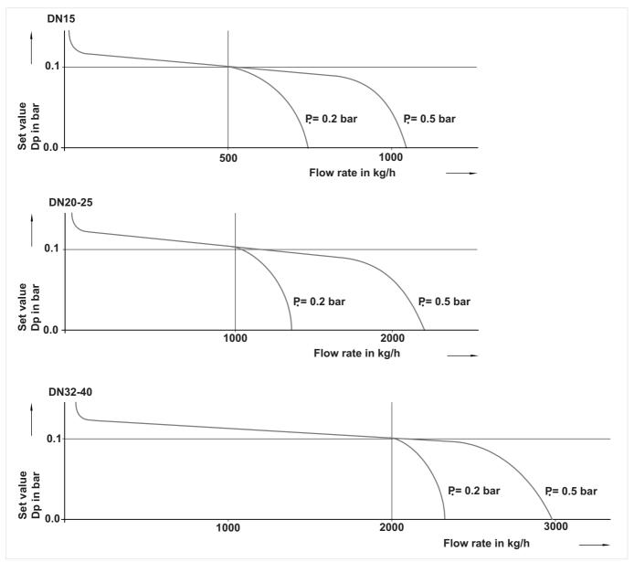
Fig. 1 Control characteristic of V5012C0103, set at 0.1 bar Dp (factory setting)
