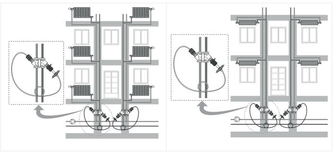
Fig. 1. V5012C Kombi-DP in a two-pipe heating system
