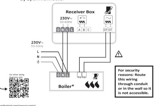
\* See boiler specifications for correct terminals
