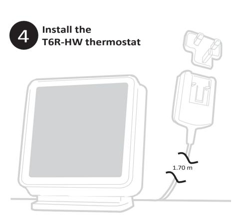
Choose the appropriate plug. Place the thermostat on an even, horizontal surface and plug it in.
