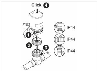
Note: Connection leads must not touch piping (heat transfer).
