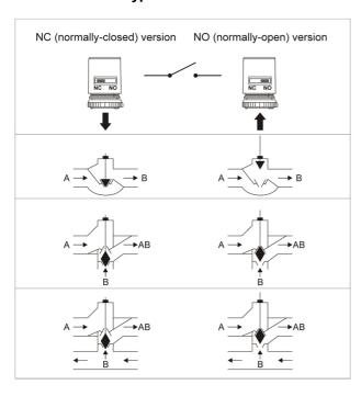
Normally open: 2-way valve, A-B open without power; Normally closed: 2-way valve, A-B shut without power;
