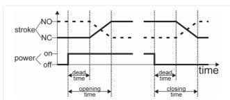
Note: Opening and closing times depend upon ambient temperature and model.
