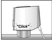
Fig. 6 Step 4: Pressing down actuator onto valve adapter
