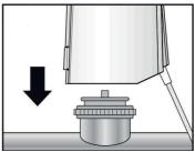
Fig. 5 Step 3: Manually positioning actuator
