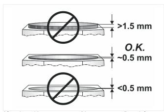
After the calibration process (drive is stopped), and if no control signal is applied, you can check whether the correct valve adapter is mounted.
