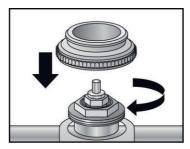
Fig. 3 Step 1: Manually screwing the adapter onto valve
