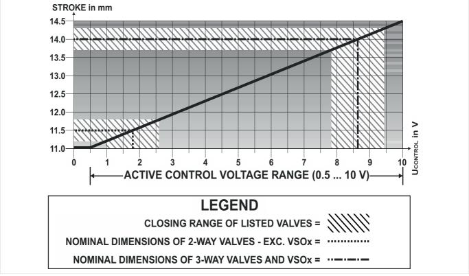
Fig. 8 Characteristic (stroke vs. voltage)
